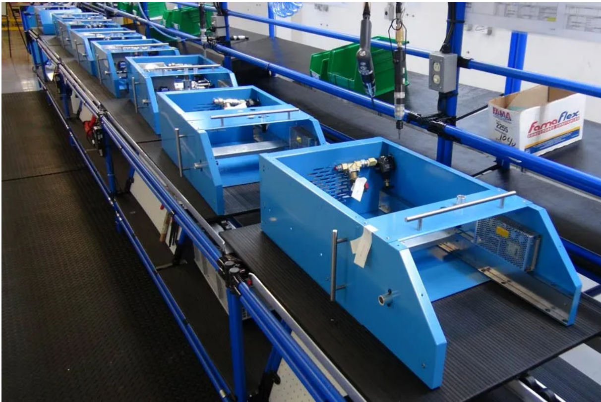
Ventilator housings on the production line.
